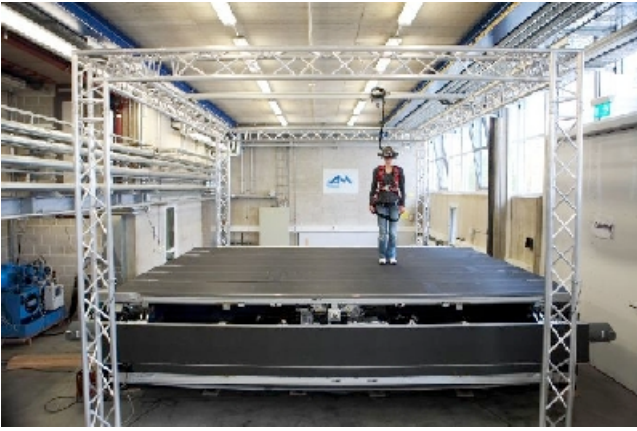
Fig. 3. The realized 2D CyberWalk platform before it was moved to its final location in Tübingen (picture courtesy of TUM, Munich)
